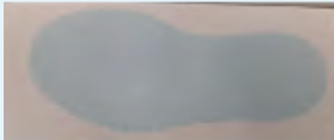
Fig. 4 Printing process of the hybrid adhesive formulation (top) Printing results on a microfibre fleece showing exemplary a common glue application on a shoe sole (left) followed a glue application with individual bondlines (middle) and an example exhibiting a high degree of design freedom (right) (adhesive is coloured for better visibility) © 2021 Covestro Deutschland AG
