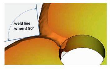
The preceding filling simulation plot shows how the flow front rejoins after splitting to pass around a hole in the plastic. A weld line will typically extend from the hole until the angle formed between the merging flow fronts exceeds about 90 degrees. The simulation was stopped at the instant when this occurred. The following image of a real part shows that the weld line does indeed extend to this location.
