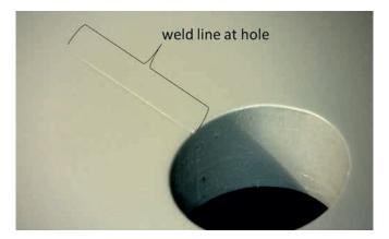
The flow front interface immediately beyond the visible weld line is called the meld line. The intermingling of polymer chains becomes increasingly improved as the meld line progresses away from the weld line until it is indistinguishable from normal flow. In glass-filled materials, the effect of the meld line on material performance may extend more than twice the length of the visible weld line. Meld lines typically have little or no effect on the performance of unfilled PC.
