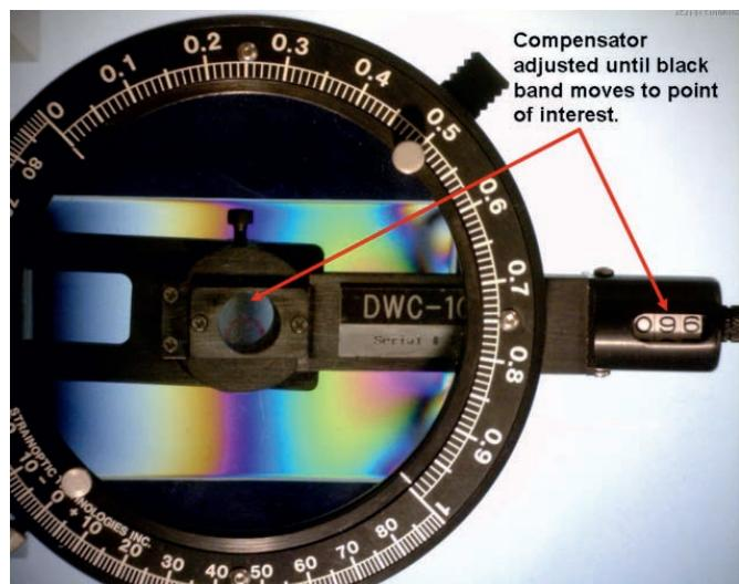
Accurate quantitative stress measurements require a polarimeter. The photo above shows a test sample in a polarimeter equipped with both a rotation analyzer, the apparatus with the circular scale, and a compensator mounted horizontally with the counter on the right and the small viewing window centered on the point of interest on the sample. Without the compensator, the rotation analyzer can be rotated to determine the fractional fringe order for calculation of the retardation.
