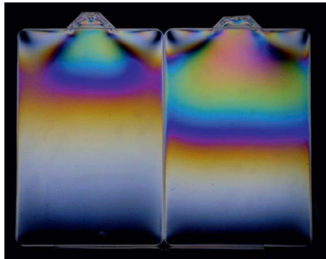
If the difference in fringe patterns can be correlated to a difference in a key part performance parameter, then this simple, non-destructive test can be used as a quality control at the molding press. Pictures of acceptable and unacceptable fringe patterns can be displayed at the press. After the parts fully cool, they can be viewed between polarizing films for a quick evaluation of molding stresses.
