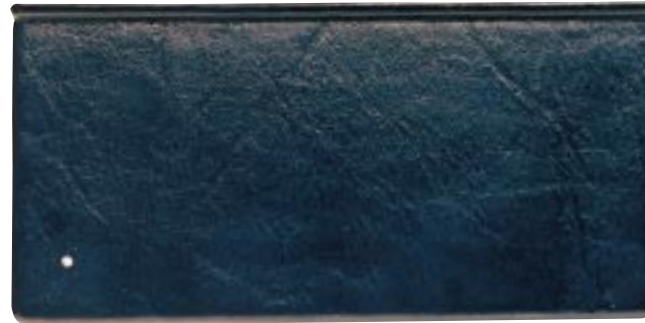
Fig. 8: Gloss difference, conditioned by the cavity wall temperature; mirror housing in ABS [5]
