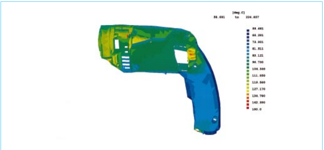
Fig. 50: Electric drill housing in polyamide PA 30 GF; computed surface temperatures on the ejector side
