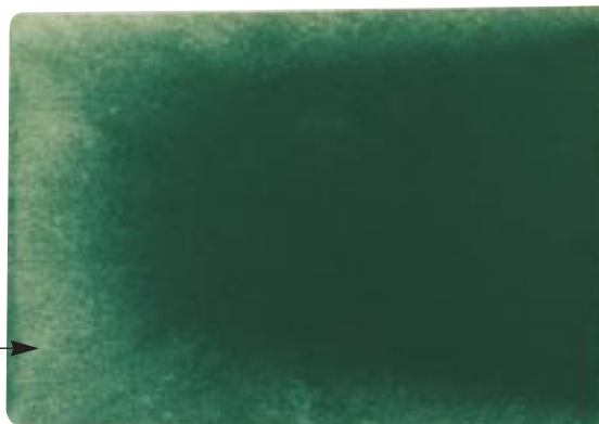
Fig. 8: Gloss difference, conditioned by the cavity wall temperature; mirror housing in ABS [5]
