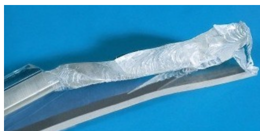
Fig. 2: Brittle fracture on a part made of hydrolytically degraded material
