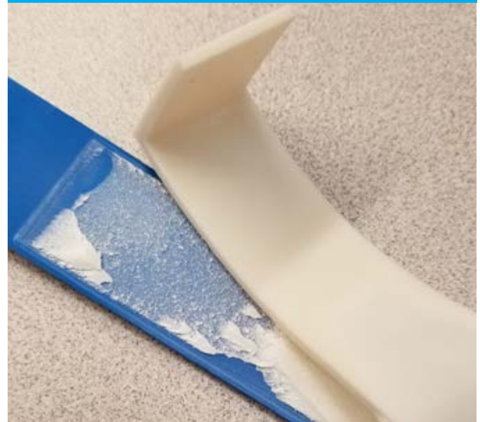
FIGURE 2 - Example of cohesive failure observed between the polycarbonates studied in this report and Medalist TPE.
