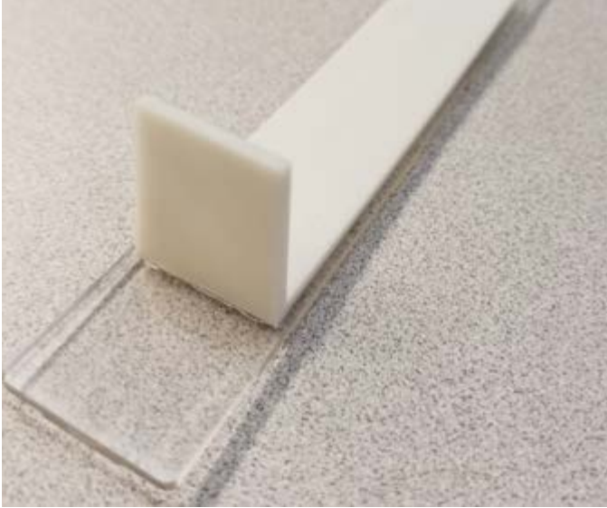
FIGURE 1 - Overmolded specimens for peel force measurements
