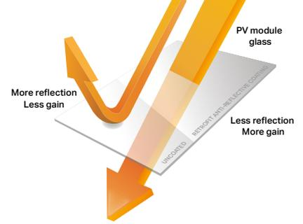
technology where we reverse the traditional nano-porous silica coating. The result is a product that is easy to clean, performs consistently – and can boost energy by up to 3%. It is applied to PV modules using a specially developed, automated spray coating system designed for optimum performance.
