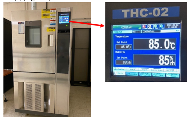
Figure 2. Damp Heat Test Setup
