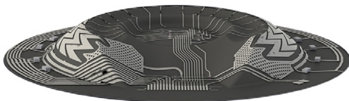
1. Film printing – decoration applied to A film, silver ink applied to B film
