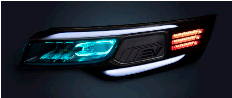
Exhibit 14 Working car headlamp concept using only polycarbonate (PC) resins
