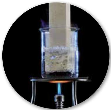
Moisture has an extreme impact on many materials. purenit retains its shape even in boiling water.
