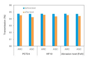
We tested sets of panels coated with Covestro Anti-Reflective coating or Covestro Anti-Soiling coating at the TÜV SÜD test site in Dunhuang, China. At this test site the Covestro Anti-Soiling coating outperformed the Anti-Reflective coating each month by ~1.1% on average.
