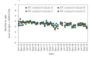
We monitor the lsc performance of up to 16 modules, measured simultaneously at five-minute intervals under maximum load in the Netherlands - which was established in partnership with Fraunhofer ISE.
