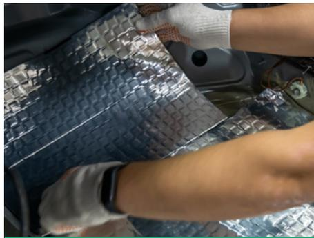
Aluminium laminate for sound absorption in cars
