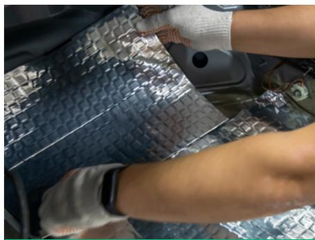
Aluminium laminate for sound absorption in cars
