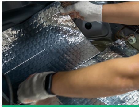
Aluminium laminate for sound absorption in cars
