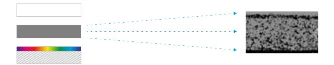
By using Makrofol® ID superlaser white, the white core section of a document allows a thinner construction by still being highly laser-reactive on both sides. This benefits in more space for overlay films and simplifies the integration of security features like chips or antennas.
