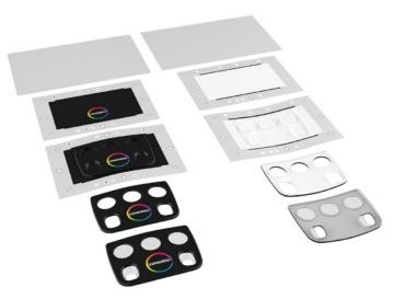
© Covestro Example of a typical FIM processing chain from a flat piece to an injection-molded functional plastic part
