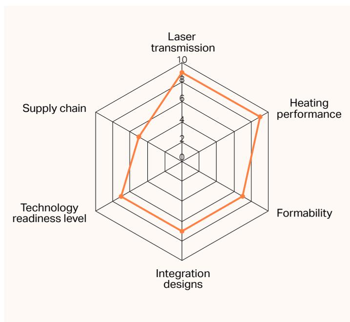
The Canatu CNT-enabled LiDAR heater received high scores on all critical parameters in Covestro's benchmark test comparing transparent heater technologies.
