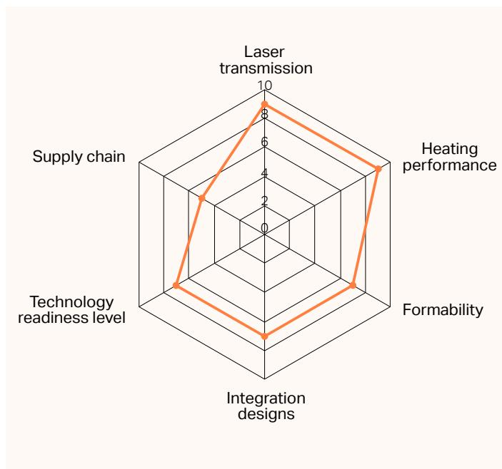
The Canatu CNT-enabled LiDAR heater received high scores on all critical parameters in Covestro's benchmark test comparing transparent heater technologies.
