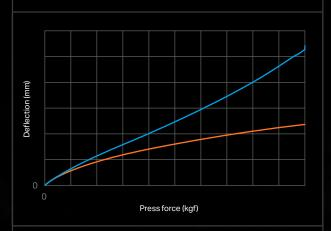
The deformation of Makrolon® high-stiffness material is only about 45% of traditional reinforced materials when under 10kg of force
