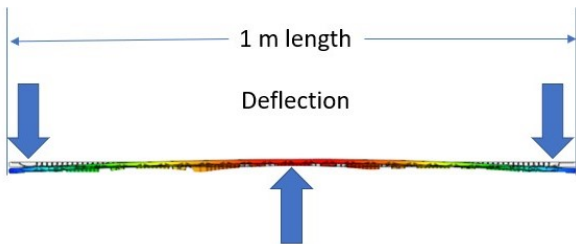
Figure 3: 1000 mm flat part warpage calculated using Bayblend® T88GF30 and 40% GF PPO/PA blend.
