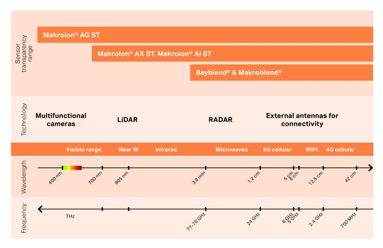
To meet the needs of this new generation of vehicles, established electronic companies are becoming increasingly active in the automotive sector. Today's cars offer more digital functions than ever before. This creates a growing need for reliable high-performance sensor-transparent materials like polycarbonates.
