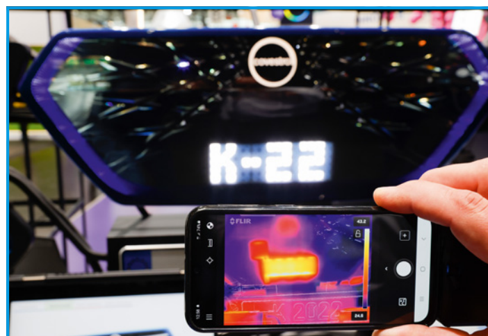
Integrated heating ensures reliable radar sensor function and display performance in harsh weather.
