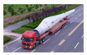
To load and secure the wind blade during transport to the place of operation, whether on the road or on a boat, the solution is to place the wind blade on cushions. Both the grip to prevent the blade from slipping and the shock resistance to absorb any shock or vibration occurring during loading and transport of the blade must be ensured.
