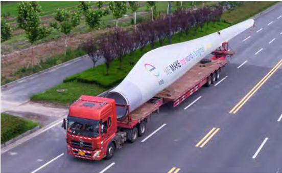
To load and secure the wind blade during transport to the place of operation, whether on the road or on a boat, the solution is to place the wind blade on cushions. Both the grip to prevent the blade from slipping and the shock resistance to absorb any shock or vibration occurring during loading and transport of the blade must be ensured.
