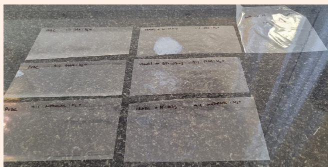
Alcohol resistance of BOPP film when coated with PVdC (left side) and Uradil FP-9300 + BT-107 (right side)
