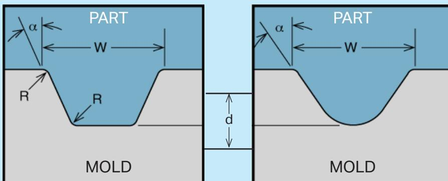
$$\alpha \geq 30^\circ \quad W \geq 2d \quad d = 0.010\text{in (max)}$$
