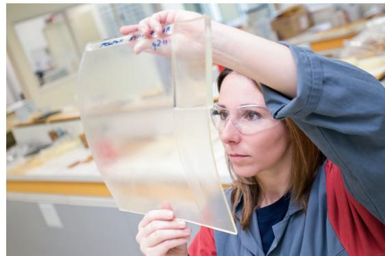
The MDI-ester quasi systems offer superior abrasion and tear resistance with excellent resistance to chemicals such as hydrocarbons, oils and solvents. It is an ideal choice for applications such as screens, scrapers, PIGs, concrete blades, sheets and vibratory bowls. The series outstanding resistance to solvents also satisfies requirements for squeegee applications.
