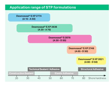
Silane-terminated polyurethanes (STP/Desmoseal® S) combine the advantages of a polyurethane backbone and a silane-based curing mechanism. That is why STPs provide a unique combination of excellent cohesive strength and good adhesive properties. We offer five **Desmoseal® S** grades covering the complete application range from low modulus sealants with very high elongation up to structural adhesives with high hardness and high tensile strength.
