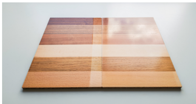
Comparison of a WB UV excimer cured wood coating (left) versus a traditional WB UV wood coating (right)
