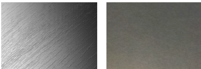
Figure 5. Different finishes possible when curing powder coatings using a press
