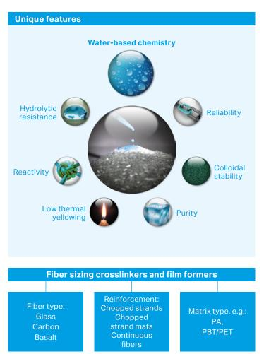
To fully exploit their ability to reinforce plastics, fibers are coated with sizing immediately after they have been manufactured. The sizing provides a chemical bond between the plastic matrix and fiber surface, key to the strength of the composite.
