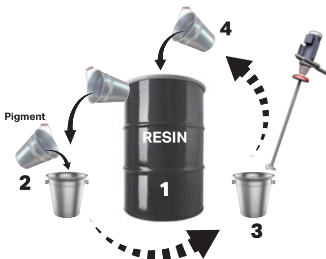
Mixing thick (high-viscosity) pigments into the resin.
