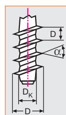
Fig. 8: Screw coupling with Apec® (recommended screw geometry)
