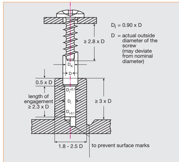
Fig. 7: Dimensioning of screw bosses for Apec®
