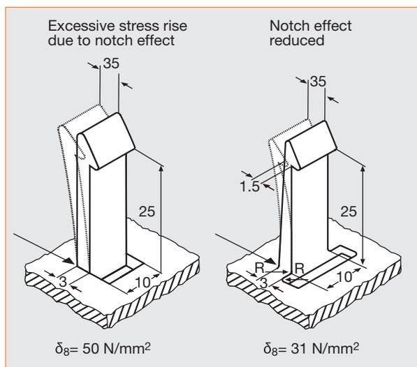
Fig. 9: Designing of snap-fit joints for Apec®
