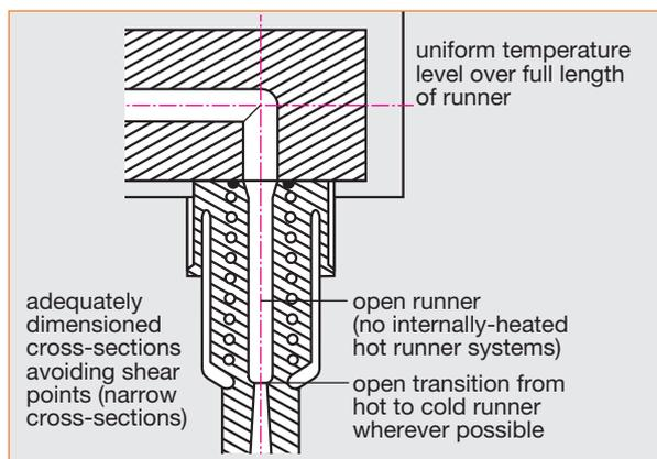
Fig. 10: Requirements for the hot runner system
