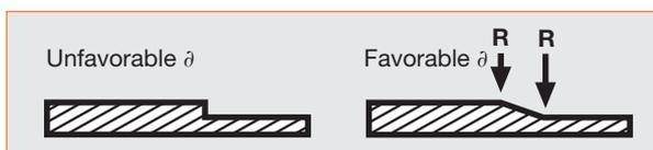
Fig. 6: Design of transitions in cross section
