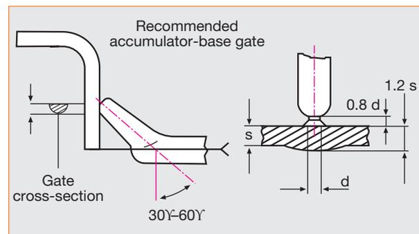
Fig. 11: Gate dimensioning – minimum gate diameter ( $d = 60\%$ ) of wall thickness ( $s$ )
