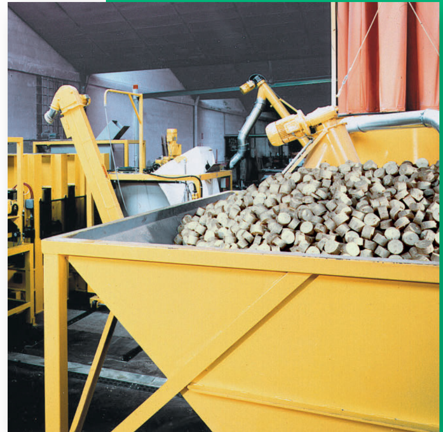
Any film or non-woven material is removed from polyurethane rigid-foam waste before it is crushed and pressed into pellets (photo: Linzmeier).
