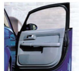
Baypreg® F: 奥迪A2汽车门板，通过天然纤维原丝毡增强 Baypreg® F: Audi A2 Door Panel, reinforced with Natural fiber mat
