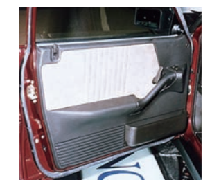
Baydur® STR: 兰吉雅汽车门板，通过磨碎玻璃或Lapinus纤维增强 Baydur® STR: Lancia Door Panel reinforced with glass or Lapinus-fibers
