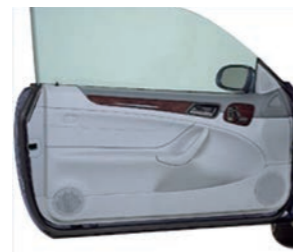
Baydur® STR: 奔驰CLK汽车门板，通过磨碎玻璃纤维增强 Baydur®STR: Mercedes CLK Door Panel reinforced with chopped glass fibers
