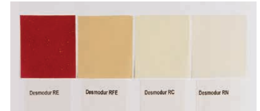
Desmodur® R: color of the dried adhesive film
