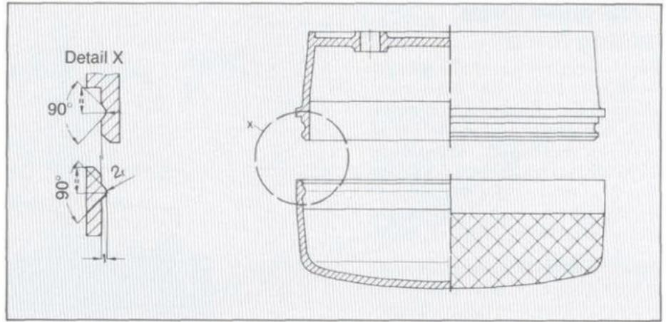
Fig. 23: Annular snap joint on a lamp housing
