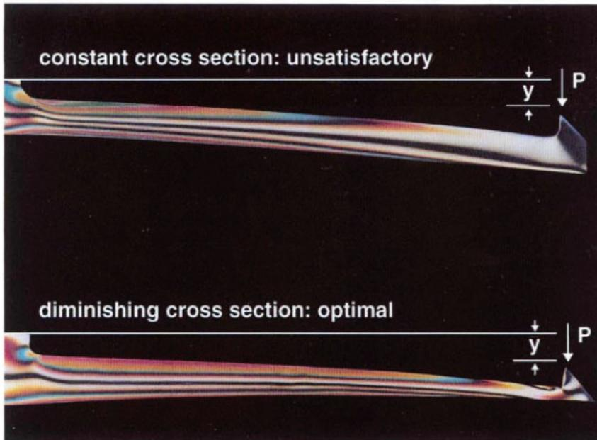
The illustration above shows a photograph of two snap-fit models taken in polarized light; both have the same displacement ( $y$ ) and deflective force ( $P$ ).
