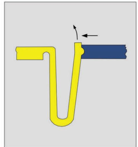
Fig. 15: U-shaped snap-fitting arm for a lid fastening
