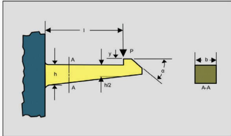
Fig. 19: Snap-fitting hook, design type 2, shape A
