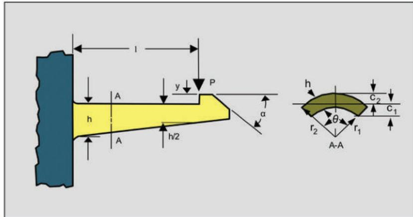
Fig. 20: Snap-fitting hook, design type 2, shape C
