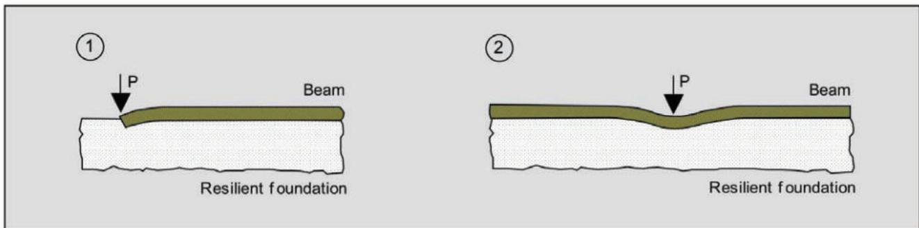
Fig. 26: Beam resting on a resilient foundation
