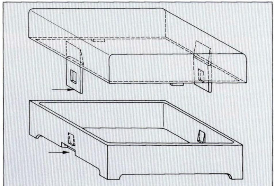
*Fig. 3: Separable snap joints for a chassis cover*
