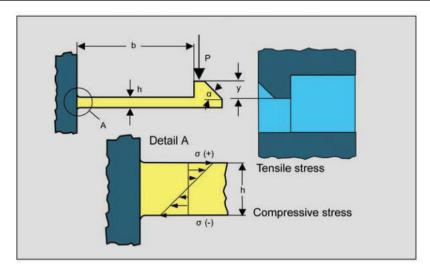
Fig. 8: Simple snap-fitting hook
