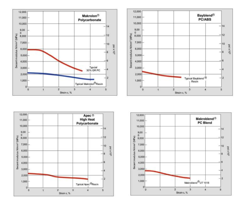
Fig. 16: Secant Modulus for Covestro engineering plastics at 23°C (73°F)
