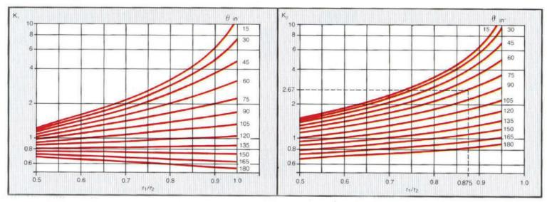
*Fig 10: Diagrams for determining K1 and K2 for cross-sectional shape type C in Table 1. K1: Concave side under tensile load, K2: Convex side under tensile load*
