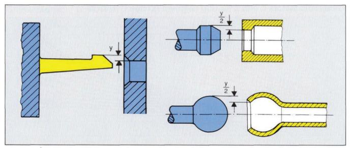
Fig 12: Undercut for snap joints
