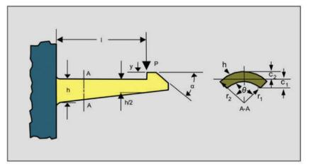
Fig. 20: Snap-fitting hook, design type 2, shape C
