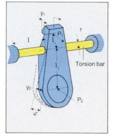
Fig. 21: Snap-fitting arm with torsion bar
