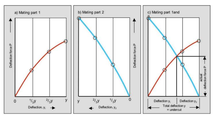
Fig. 29: Determination of deformation and transverse force when both mating parts are flexible
