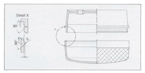
Fig. 23: Annular snap joint on a lamp housing
