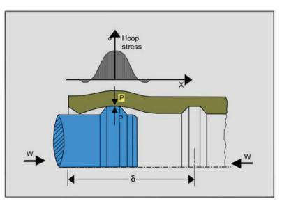
Fig. 25: Stress distribution during joining operation
