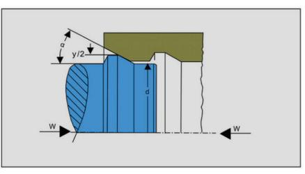
Fig. 24: Annular snap joint-symbols used
