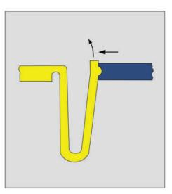
Fig. 15: U-shaped snap-fitting arm for a lid fastening
