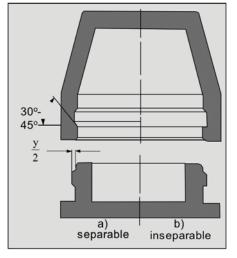
Fig. 22: Annular snap joint
