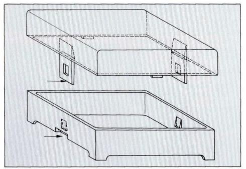
Fig. 3: Separable snap joints for a chassis cover
