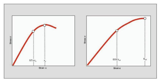
Fig 13: Determination of the permissible strain for the joining operation (left: material with distinct yield point; right: glass-fiber-reinforced material without yield point)
