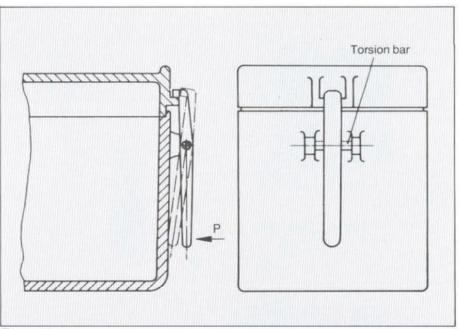
Fig 5: Torsion snap joint on a housing made of Makrolon<sup>®</sup> polycarbonate
