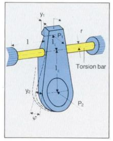
Fig. 21: Snap-fitting arm with torsion bar
