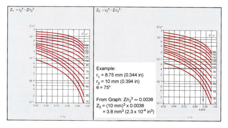
Fig 11: Graphs for determining the dimensionless quantity (Z/r23) used to derive the section modulus (Z) for cross-sectional shape C in Table 1.
