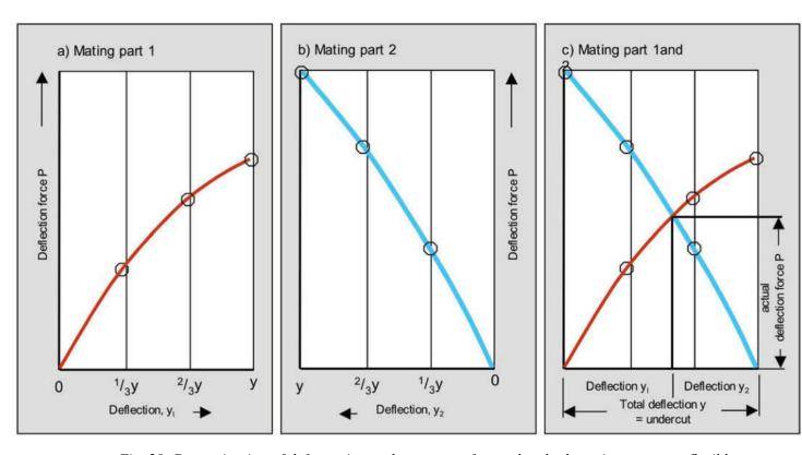
Fig. 29: Determination of deformation and transverse force when both mating parts are flexible
