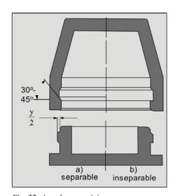
Fig. 22: Annular snap joint
