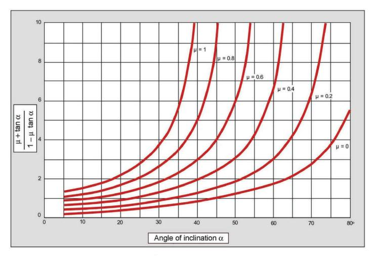
Figure 18: Diagram for determining  $\mu + \tan \alpha$ 1 –  $\mu \tan \alpha$
