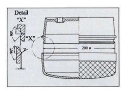
Fig. 28: Lamp housing with cover
