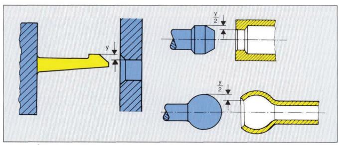
Fig 12: Undercut for snap joints
