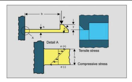
Fig. 8: Simple snap-fitting hook
