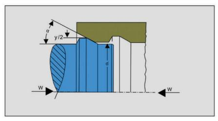
Fig. 24: Annular snap joint—symbols used
