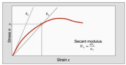
Fig. 14: Determination of the secant modulus
