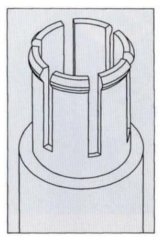
Fig. 1: Module for control panels with four cantilever lugs
