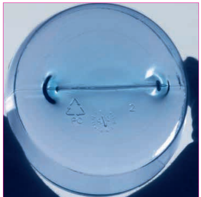
Fig. 4: Base of bottle, annealed after cleaning
