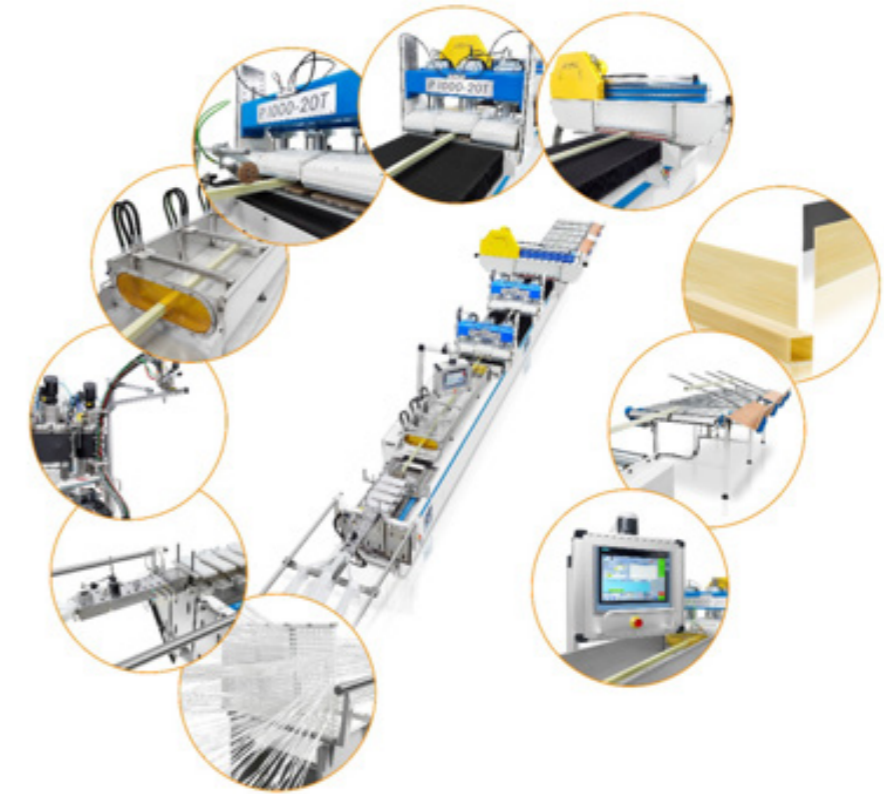
Fig. 3 Polyurethane pultrusion line (KraussMaffei Technologies GmbH)
