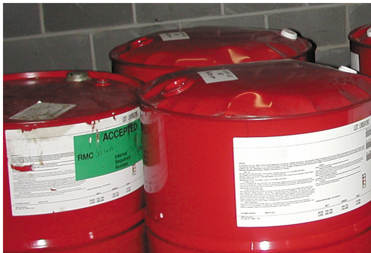
Figure 1 - Swollen drums are potentially dangerous
