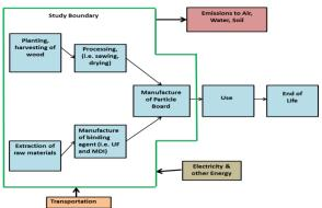
System boundary of the particle board
