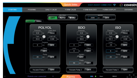
Human-Machine interface: process information display
